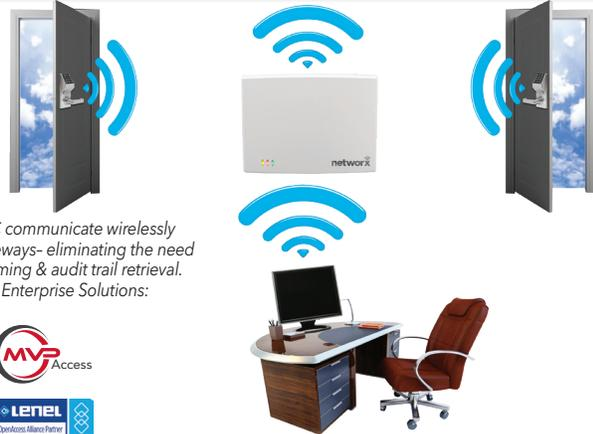
Up to 2000 locks and a PC communicate wirelessly through bidirectional Gateways- eliminating the need for door-to-door programming & audit trail retrieval. System Management with Enterprise Solutions:
